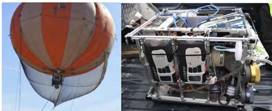
Fig. 2. Aerostat with Flyer (Left) and Flyer close up (Right).
